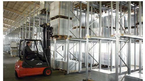
Smooth pallet rails provide a safe, snag-free load-bearing surface. The rails are carried on brackets that slot into the uprights. Like regular beams, they're adjustable to 50mm, and secured with an automatic safety lock. Brightly coloured pallet guides help drivers position loads quickly and accurately.
